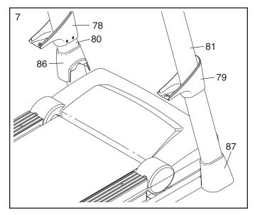
Cut the plastic tie in the Left Handrail (84) and the Right Handrail (85). If necessary, press the 5/16" Cage Nuts (31) back into place.
